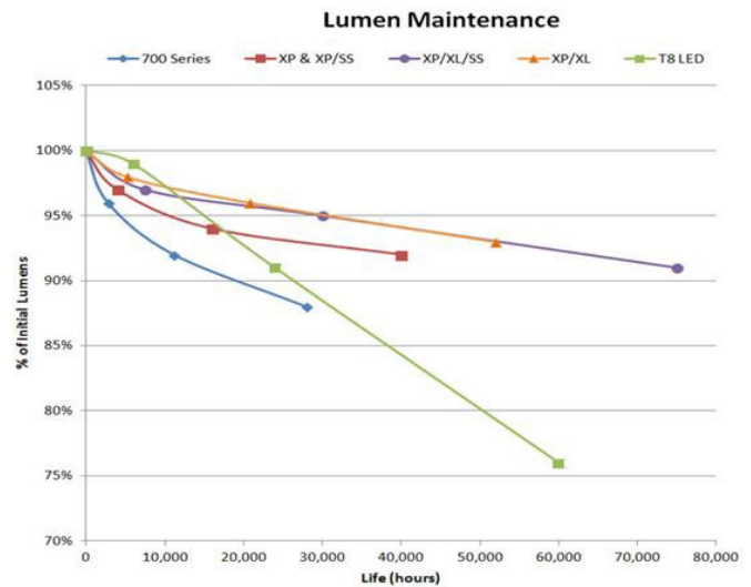
FIGURE 1-13 Lamp lumen depreciation curves for common lamp types. Courtesy of OSRAM SYLVANIA.
